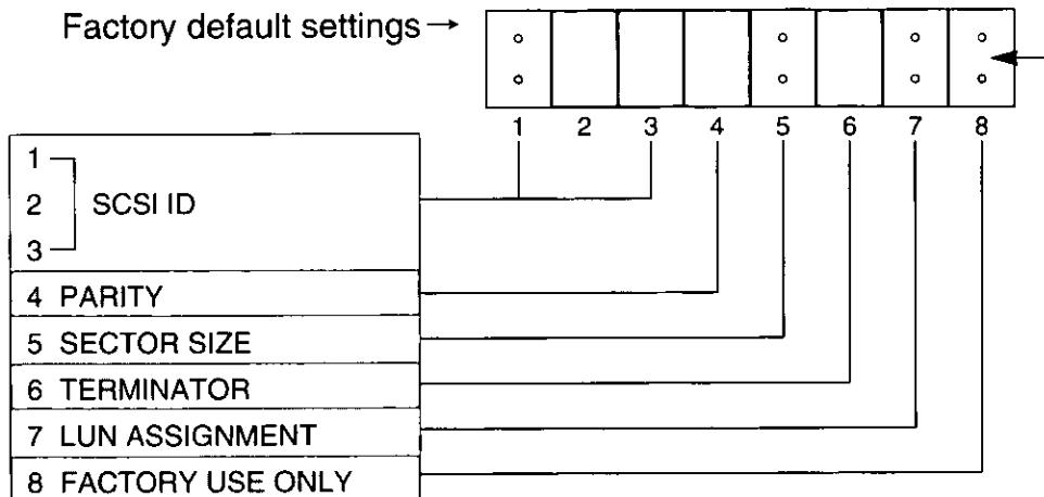
To change the setting, pull the jumper off with tweezers and slide the jumper onto the correct pins.
