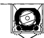
Keep the latches on the adapter to the bottom when fitting it into the tray.
